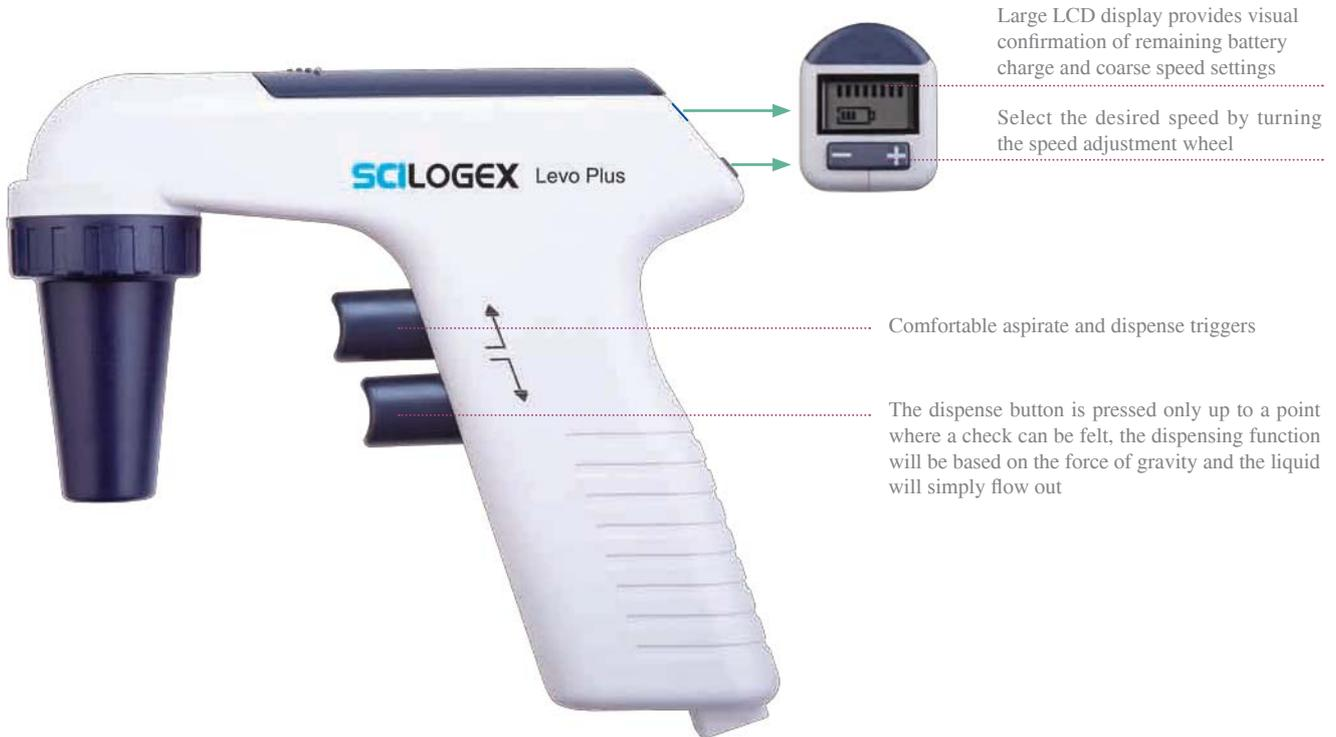
Large LCD display provides visual confirmation of remaining battery charge and coarse speed settings
