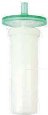
The 0.45µm filter and adapter can be integral and replaceable
